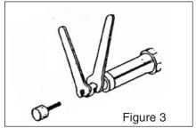
Note: Before each use, always check that the mandrel is securely fastened into the Collet Chuck (#1).
